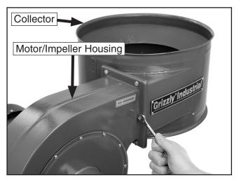
**Figure 8.** Installing collector onto motor/impeller housing.
